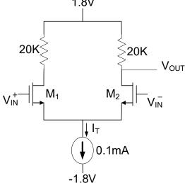
Problem 7 (10 points) Consider the operational amplifier where the resistors are ideal and where the transistors are biased for  $V_{EB}$ =0.25V.
